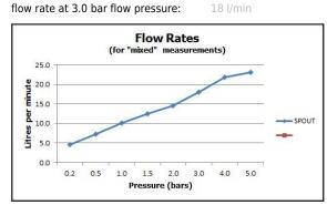
'mixed measurements' refers to equal hot and cold water supply flow rate for unregulated flow unless flow regulator fitted as standard
