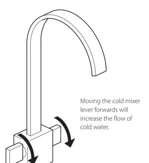
Moving the hot mixer lever forwards will increase the flow of hot water.
