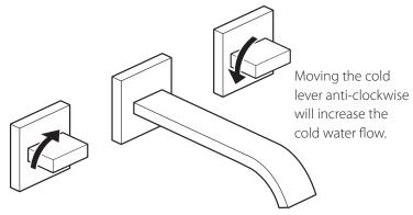
Moving the hot lever clockwise will increase the hot water flow
