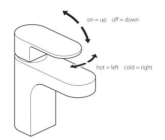
Moving the mixer lever upwards/downwards will increase/decrease the flow of water. Moving the mixer lever from right to left will increase the water temperature.
