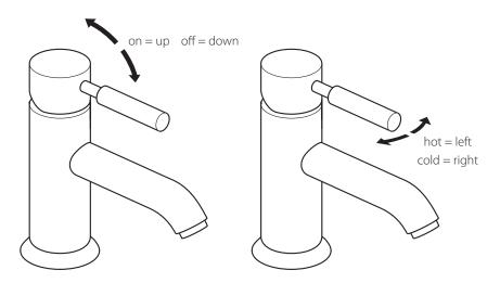
Moving the mixer lever upwards/downwards will increase/decrease the flow of water. Moving the mixer lever from right to left will increase the water temperature.
