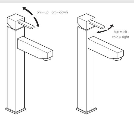
Moving the mixer lever upwards/downwards will increase/decrease the flow of water. Moving the mixer lever from right to left will increase the water temperature.
